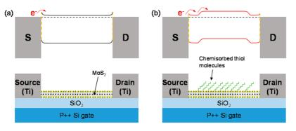
Figure 8. Schematics of the energy band diagram at  $V_{G} = 0$  (a) before and (b) after the alkanethiol molecule treatment.
