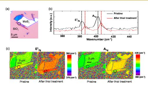
Figure 5. (a) Optical image of a  $MoS_2$  flake that was used for Raman and PL studies. (b) Raman spectra measured from a circled region marked in (a) before and after the hexadecanethiol treatment. (c) Raman mapping image of the  $E^{1}_{2g}$  mode and  $A_{1g}$  mode before (left) and after (right) the hexadecanethiol treatment. We added dotted lines to indicate the  $MoS_2$  flakes in this figure.
