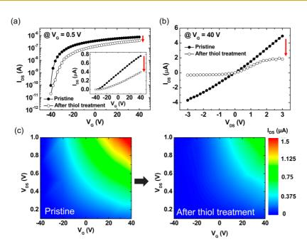
Figure 3. (a)  $I_{DS}-V_G$  curves measured before and after the hexadecanethiol treatment with logarithmic scale. The inset shows  $I_{DS}-V_G$  curves with linear scale. (b)  $I_{DS}-V_{DS}$  curves measured before and after the hexadecanethiol treatment. (c) Contour plots of  $I_{DS}$  as a function of  $V_G$  and  $V_{DS}$  before (left) and after (right) the hexadecanethiol treatment.
