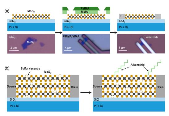
Figure 1. (a) Schematic images of the fabrication process of  $MoS_2$  FETs with the optical images shown under each schematic image. (b) Schematic images of a  $MoS_2$  FET before (left) and after (right) the alkanethiol molecule treatment.
