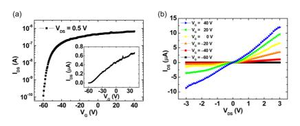
Figure 2. (a)  $I_{DS}-V_G$  curve measured at a fixed  $V_{DS} = 0.5$  V with logarithmic scale. The inset shows  $I_{DS}-V_G$  curves with linear scale. (b)  $I_{DS}-V_{DS}$  curves measured with  $V_G$  varying from 40 to -60 V.
