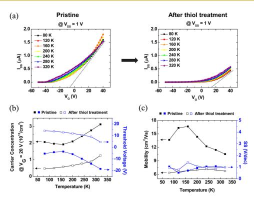
Figure 4. (a) I<sub>DS</sub>-V<sub>G</sub> curves measured before and after hexadecanethiol treatment with varying temperatures from 80 to 320 K. (b) Carrier concentration and threshold voltage of a MoS<sub>2</sub> FET as a function of temperature acquired before and after the hexadecanethiol treatment. (c) Mobility and SS value of a MoS<sub>2</sub> FET as a function of temperature acquired before and after the hexadecanethiol treatment.
