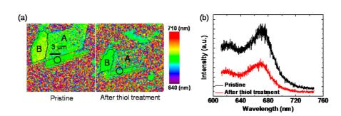
Figure 6. (a) PL peak position mapping image of the  $MoS_2$  flake shown in Figure 4a before (left) and after (right) the hexadecanethiol treatment. (b) PL spectra measured from a circled region before and after the hexadecanethiol treatment. We added dotted lines to indicate the  $MoS_2$  flakes in this figure.
