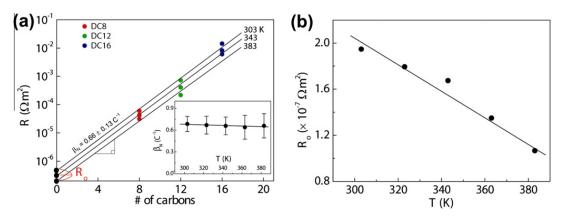
**Fig. 4**. (a) A plot of resistance *R* versus the number of molecular carbons of DC8, DC12, and DC16 PEDOT:PSS-interlayer molecular junctions. The solid lines are the exponential fitting results, which give  $\beta_N$  as a function of the annealing temperature (inset). The *y*-intercept points are the effective contact resistance  $R_0$ . (b) A plot of  $R_0$  versus the annealing temperatures.
