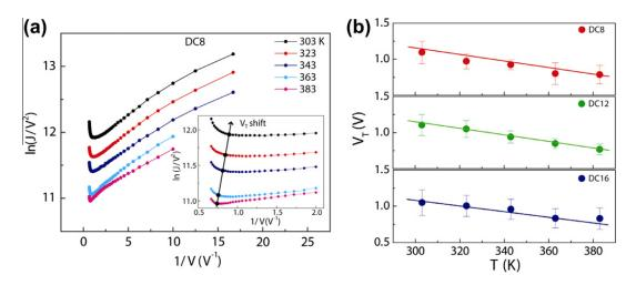
**Fig. 6.** (a)  $\ln(J/V^2)$  versus 1/V curves for DC8 PEDOT:PSS-interlayer molecular junctions measured at different temperatures (303–383 K, 20 K step). Inset is a zoomed-in plot near the transition voltages  $V_T$  (minimum points of the curves). (b) Experimental  $V_T$  for DC8, DC12, and DC16 PEDOT:PSS-interlayer molecular junctions in the temperature range from 303 to 383 K.
