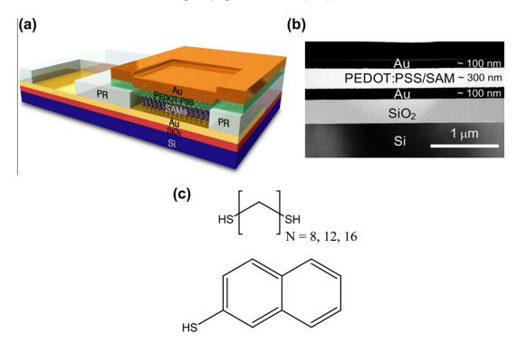
**Fig. 1.** (a) Schematic illustration of a PEDOT:PSS-interlayer molecular junction. (b) The cross-sectional TEM image in the active region for a molecular device. (c) The N-alkanedithiols and naphthalenethiol molecular structures are shown.
