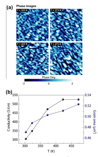
**Fig. 5.** (a) The AFM phase images of  $1 \times 1 \ \mu\text{m}^2$  regions of 7% DMSO-modified PEDOT:PSS films at different annealing temperatures (323–473 K, step 50 K). (b) Temperature dependence of conductivity and grain area for 7% DMSO-modified PEDOT:PSS films.
