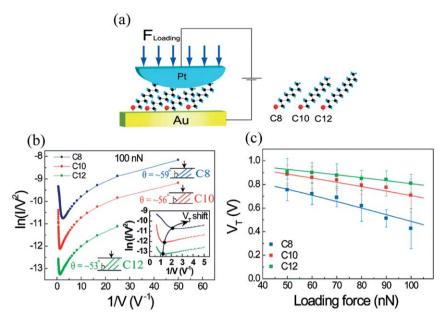
Fig. 17 (a) Schematic of a molecular junction using the CP-AFM method. C8, C10, and C12 molecular structures are shown (right). (b) The plot of  $IIV^2$ ) versus IIV for C8, C10, and C12 at a fixed tip-loading force of 100 nN. Insets show that the transition voltage IIV from DT to F-N occurs at a lower bias for shorter molecules. (c) Experimental IIV versus tip-loading force for C8, C10, and C12 molecular junctions. Reprinted with permission from ref. 170, © 2009, American Chemical Society.
