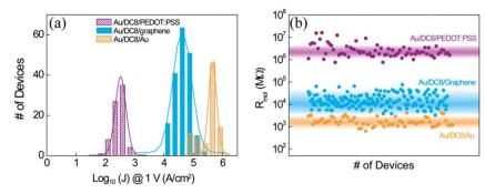
Fig. 5 (a) Histogram of logarithmic J at 1 V for molecular devices with different types of top electrodes (PEDOT:PSS, graphene, or Au). (b) The resistance per molecule  $R_{\text{mol}}$  values for these molecular junctions. Reprinted with permission from ref. 44, © 2011, Wiley-VCH Verlag GmbH & Co. KGaA, Weinheim.
