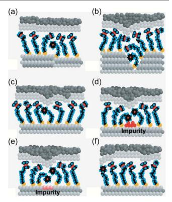
Fig. 2 Schematic of several possible defects in Ga<sub>2</sub>O<sub>3</sub> interlayer-based molecular junction: (a) step edges and vacancy island on bottom electrode surface, (b) grain boundaries on bottom electrode surface, (c) different orientation of the molecular chains, (d) and (e) impurities in bottom electrode surface, and (f) non-conformal contact of the top electrode with the SAM. Reprinted with permission from ref. 135, © 2010 American Chemical Society.
