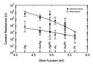
Fig. 8 Contact resistance  $R_0$  as a function of electrode metal work function for alkanemonothiols (●) and alkanedithiols (○) in CP-AFM junctions. Reprinted with permission from ref. 94, © 2004, American Chemical Society.
