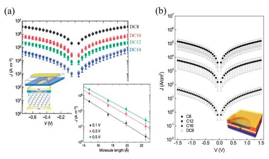
Fig. 4 (a) The J-V characteristics for the PEDOT:PSS-based alkanedithiol (DC8, DC10, DC12, and DC14) junction. The inset shows the J-d (molecular length) plot in the low bias region. Reprinted with permission from ref. 37, © 2006, Nature Publishing Group. (b) The J-V characteristics for graphene-based alkanedithiol (DC8, DC12, and DC16) and alkanemonothiol (C8) junctions. Reprinted with permission from ref. 44, © 2011, Wiley-VCH Verlag GmbH & Co. KGaA, Weinheim.
