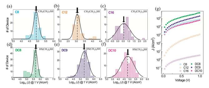
Fig. 3 Statistical histograms of  $\log J$  measured at 1.0 V for (a) C8, (b) C12, (c) C16, (d) DC8, (e) DC9, and (f) DC10. The line curves are fitted results obtained from the histograms with Gaussian functions and the mean positions are indicated with arrows. (g) J-V characteristics of representative devices chosen from the mean positions of the fitted Gaussian function. Reprinted with permission from ref. 55, © 2007, The American Physical Society.
