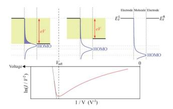
**Fig. 14** The scenario for the inflection in the F–N curve. The shaded area indicates the electric current magnitude at  $V_{\rm infl}$  ( $V_{\rm T}$ ). Reprinted with permission from ref. 61, © 2010, The American Physical Society.
