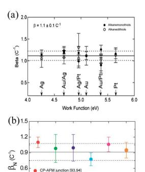
Fig. 7 (a) The  $\beta$  values as a function of electrode metal work functions for alkanemonothiols (●) and alkanedithiols (○) in a CP-AFM junction. Reprinted with permission from ref. 94, © 2004, American Chemical Society. (b) The  $\beta$  values of alkyl-based molecular junctions in different testbeds. 37,43,44,55,86,87,93,94,109,148
