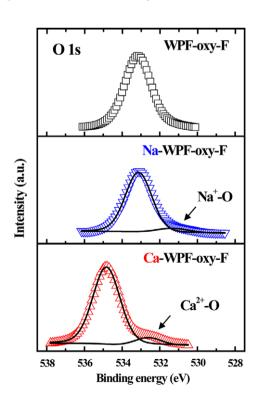
**Fig. 2.** XPS spectra of oxygen 1s peaks for WPF-oxy-F, Na-WPF-oxy-F and Ca-WPF-oxy-F.
