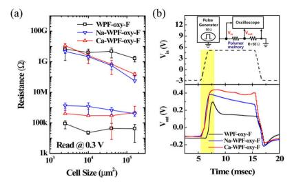
**Fig. 6.** (a) Resistance values of the on and off states of the three kinds of polyfluorene-derivative memory devices as a function of junction area. (b) Transient response characteristics of the three kinds of polyfluorene-derivative memory devices. The inset shows the circuit of measurement method.
