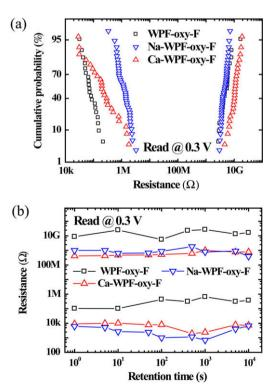
**Fig. 4.** (a) A Cumulative probability data sets of WPF-oxy-F, Na-WPF-oxy-F and Ca-WPF-oxy-F. (b) Retention characteristics of WPF-oxy-F, Na-WPF-oxy-F and Ca-WPF-oxy-F measured at room temperature.
