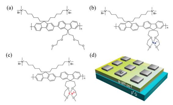
Fig. 1. Chemical structures of polyfluorene-derivatives (a) WPF-oxy-F, (b) Na-WPF-oxy-F and (c) Ca-WPF-oxy-F. (d) Schematic of MIM-type organic non-volatile memory device.
