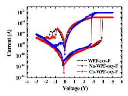
Fig. 3. Semi-log scale  $\it I-V$  characteristics of WPF-oxy-F, Na-WPF-oxy-F and Ca-WPF-oxy-F with a cell size of 50  $\times$  50  $\mu m^2.$
