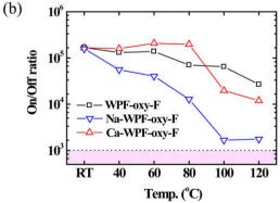
**Fig. 5.** (a) Distributions of threshold voltage of organic non-volatile memory devices with WPF-oxy-F, Na-WPF-oxy-F and Ca-WPF-oxy-F. Inset shows the histogram of threshold voltage for Na-WPF-oxy-F. (b) Comparisons of on/off ratios of three kinds of polyfluorene-derivatives measured at various temperatures.
