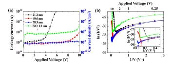
FIG. 3. (Color online) (a) Leakage current density vs applied voltage through  $Al_2O_3$  dielectric layers of different thicknesses (21.2, 49.6, and 78.3 nm) and a 12 nm SiO<sub>2</sub> layer. (b)  $ln(I/V^2)$  vs 1/V plot for  $Al_2O_3$  and 12 nm SiO<sub>2</sub> dielectric layers. Inset is a zoomed-in plot near the transition voltages (marked by arrows) from DT to FN tunneling (see text in detail).
