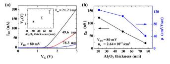
FIG. 4. (Color online) (a)  $I_{DS}-V_G$  characteristics for ZnO nanowire FETs with varying  $Al_2O_3$  dielectric thicknesses at fixed  $V_{DS}$ =80 mV. The inset shows the statistical distribution of the measured threshold voltage. (b) Transconductance ( $g_m$ ) and mobility ( $\mu$ ) of ZnO nanowire FETs with varying  $Al_2O_3$  dielectric thicknesses.
