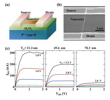
FIG. 2. (Color online) (a) Schematic of a ZnO nanowire FET device structure. (b) Scanning electron microscopy image of a single ZnO nanowire connected between source and drain electrodes in a FET device. (c) A series of  $I_{DS}-V_{DS}$  characteristics for ZnO nanowire FETs with varying  $Al_2O_3$  dielectric thicknesses (21.2, 49.6, and 78.3 nm).
