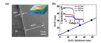
FIG. 1. (Color online) (a) HRTEM image of  $Al_2O_3$  dielectric layer (21.2 nm). The inset shows schematic of a MOS device structure. (b) EOT vs thickness of  $Al_2O_3$  dielectric layer. The inset shows a series of C-V characteristics.
