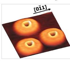
480×480 nm atomic force microscopy image of a typical CRD.
