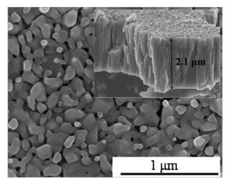
Scanning electron microscopy (SEM) images of WO<sub>3</sub> layers after annealing at 450 °C in air for 1 h followed by a NH<sub>3</sub> treatment at 600 °C. The treatment time is 4 h for all the samples. The inset shows a cross-sectional SEM image.
