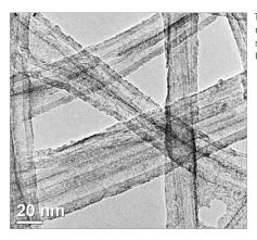
Transmission electron microscopy image of several CNTs covered with a layer of NiO nanoparticles.
