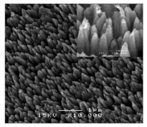
Scanning electron microscopy image of an Au nanoneedle array prepared by an Au film with a thickness of 400 nm. The inset is the high-resolution SEM image of several Au nanoneedles observed at a tilt angle of 45°.
