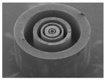
Scanning electron microscopy image of three-dimensional microstructures etched in silicon covered with nickel-coated TMV.
