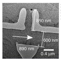
An image of the heating element used to form gold clusters. The arrow shows the direction the current will flow when applied.
