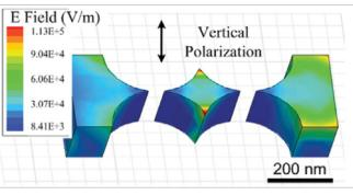
Electrical field distribution within the electrodes with the laser beam polarization normal to the electrode tip pair.
