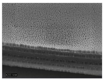
Multi-layer TiO<sub>2</sub> structure. (Note: The multi-layer structure in the picture was produced accidentally. We are still looking for a method to consistently reproduce the multi-layer structure. But this accident gives strong evidence that the multi-layer structure can be very sturdy and its fabrication is highly possible.)
