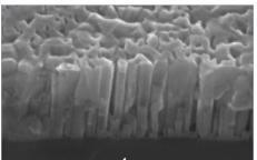
Scanning electron microscopy image showing a continuous GaN:Mg top contact layer grown on GaN nanowires.
