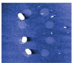
Lateral force microscopy image of DPN-generated MHA-PLL dot patterns after the addition of *E. coli* K12 bacteria.
