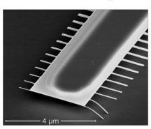
Series of freestanding cantilevers on (100) Si substrate. The implantation dose was  $4 \times 10^{15}$  ions cm<sup>-2</sup>. The length of the cantilevers is  $0.5\,\mu$ m (left) and  $1\,\mu$ m (right), the thickness approx. 50 nm and the width of the narrowest beams 35 nm. The two bridges adhere to the substrate because of stiction deriving from the drying step of the wet release process.
