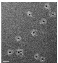
Transmission electron microscopy image of a conjugate of TFG protein and gold nanoparticles. Sample was stained by 3% phosphotungstic acid. Bar size: 20 nm.
