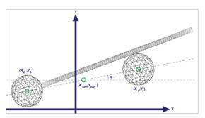
A schematic of the fabricated nanotool is shown. The coordinate system (x, y) is defined such that the average position of the tool is equal to zero,  $\langle x_{tool'}, \varphi_{too} \rangle = (0, 0, 0)$ . The green circles represent the location of the relevant coordinate, and the subscripts refer to the position of the tool, microsphere 0, or microsphere 1.  $\theta_{tool}$  is the angle of the tool, relative to the x-axis.
