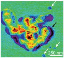
MFM phase shift images at lift heights of 15 nm containing a cluster of  $Fe_3O_4$  NPs (black arrow) and scattered AuNPs (some examples with white arrows).
