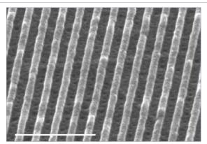
Scanning electron microscopy image of 200 nm period metal gratings in nickel patterned by LADI with a laser fluence of 0.41 J cm  $^{-2}$ . Scale bar is 1  $\mu$ m.
