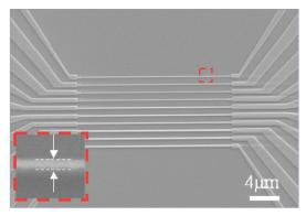
Silicon nanowire sensor arrays fabricated by the top-down nanofabrication process (inset:  $50\,\text{nm}$  width).
