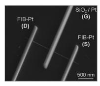
Scanning electron microscopy image of an enhancement-mode FET device on a ZnO nanowire. The source [S] and drain [D] electrodes were fabricated by FIB-deposited Pt, while the gate [G] Pt electrode is lying on an *in situ* deposited SiO<sub>2</sub> layer on the ZnO nanowire surface.
