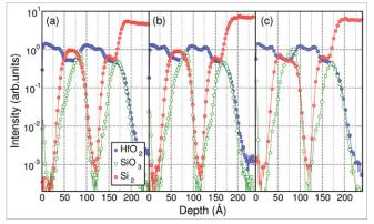
ToF-SIMS profile of the Hf0\_/4 nm thick SiO/Hf0\_ multilayer structure without SiO\_ capping layer before (a) and after thermal treatment at 600 °C (b) and 900 °C (c) in N<sub>2</sub> atmosphere for 60 min. The intensity of the Si<sub>2</sub> signal at the surface increases with the annealing temperature.
