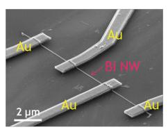
Scanning electron microscopy image of fourprobe device based on an individual Bi nanowire to investigate its transport properties.
