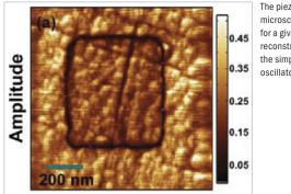
The piezoresponse force microscopy amplitude for a given frequency reconstructed from the simple harmonic oscillator fit parameter.
