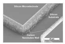
Scanning electron microscopy image of the silicon microelectrode, silicon substrate, and CNT wall.
