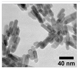
Transmission electron microscopy image of the ZnO nanorod sample  $13\times 50\,\text{nm}$  synthesized from solution.
