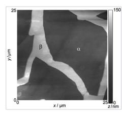
SECM-SFM topographical image of a coarse-grained Ti-6AI-4V specimen in a solution of 2 mM [Ru(NH<sub>3</sub>)<sub>6</sub>]Cl<sub>3</sub> in 0.1 M KCI. The image was scanned from right to left
