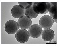
Transmission electron microscopy image showing gold shell growth using LPS@C18N3@Au seed.
