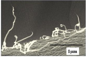
Scanning electron microscopy image of a SWNT surface with occasional protruding tubes created during deposition or film handling.
