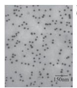
Transmission electron microscopy image of the 16 nm Cys-GNPs.
