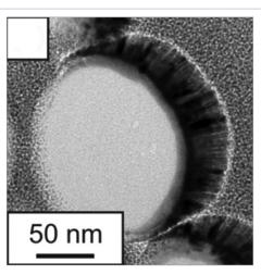
Cross-sectional transmission electron microscopy image of a magnetic cap grown on a 160 nm SiO<sub>2</sub> particle.
