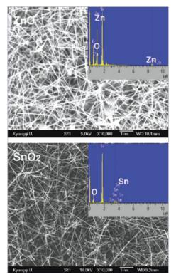
Field-emission scanning electron microscopy images of ZnO nanowires (D - 70 nm) and SnO<sub>2</sub> nanowires (D - 40 nm). The images in the inset show EDS data for ZnO and SnO<sub>2</sub>.
