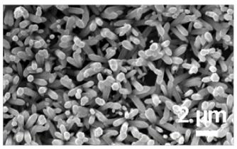
Top-view scanning electron microscopy image of ZnO nanorod array obtained by passing a charge density of  $2.5\,$  Ccm<sup>-2</sup>.
