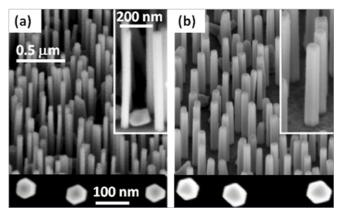
Scanning electron micrographs of InAs nanowires grown on Si(111) at temperatures of (a) 430 °C and (b) 505 °C. Magnified areas (insets) and top-view images (bottom) show the nanowire/substrate interface and hexagonal geometry, respectively.
