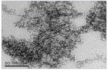
High-resolution transmission electron microscopy image of CdTe QDs.
