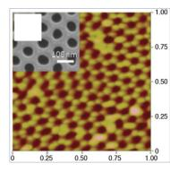
Atomic force microscopy image of alumina template as a function of pore sizes, in this case 50 nm. Inner square shows a scanning electron microscope image.
