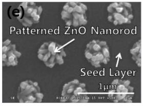
Scanning electron micrograph of a selectively grown ZnO nanorod array on the ITO electrode after removing the imprinted polymer pattern.
