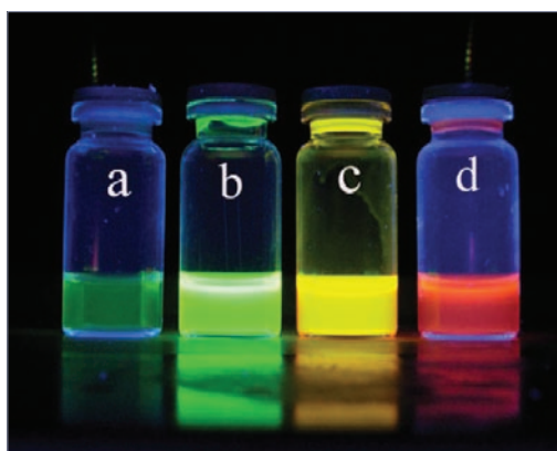
Photograph of the wide spectral range of bright luminescence from the sample of CdTe core QDs (a) and CdTe/CdSe QDs ((b)-(d)) dispersed in water.
