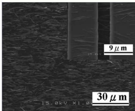
Scanning electron micrograph images of roll-transferred ZnO nanowires. Source and drain electrodes are deposited following the transfer.
