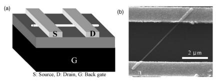
Fig. 2. (a) Schematic structure of ZnO nanowire FET. (b) FESEM image of ZnO nanowire FET.
