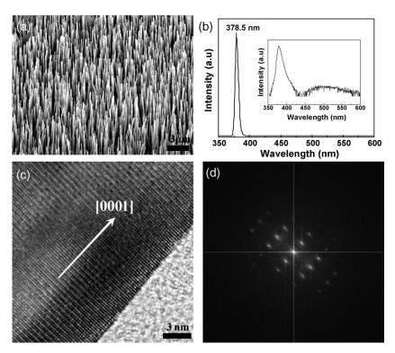
Fig. 1. (a) FESEM image (tilted view) of the ZnO nanowires grown on the sapphire substrate. (b) PL emission spectrum showing a strong emission at approximately 378.5 nm. The inset shows the logarithmic-scale plot. (c) HRTEM image of an individual ZnO nanowire showing its [0 0 0 1] growth direction. (d) The faster Fourier transform pattern corresponding to the lattice fringes from the nanowires.
