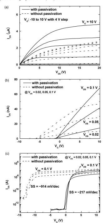
Fig. 3. (a) Source–drain current vs. voltage  $(I_{\rm DS}-V_{\rm DS})$  characteristics at different gate voltages with and without passivation, (b) source–drain current vs. gate voltage  $(I_{\rm DS}-V_{\rm G})$  characteristics at different source–drain biases for the same ZnO nanowire FET, respectively. (c) Logarithmic plot of  $I_{\rm DS}-V_{\rm G}$  curves at  $V_{\rm DS}=0.02$ , 0.05, and 0.1 V for another ZnO nanowire FET device.
