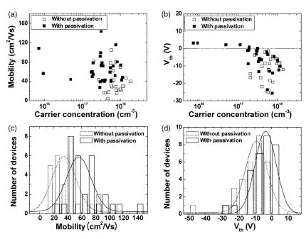
Fig. 4. (a) Mobility vs. carrier concentration and (b) threshold voltage ( $V_{th}$ ) vs. carrier concentration for all ZnO nanowire FETs fabricated. Histogram of threshold voltages (a) and mobility (b) for the ZnO nanowire FETs with and without passivation.
