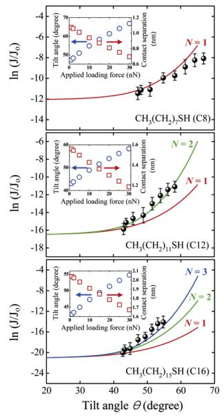
**Figure 1.** Semilog plots of normalized tunneling current densities as a function of the molecular tilt angle for different length alkanethiols. Insets show the relationship of molecular tilt angle  $\theta$ , contact separation, and tiploading force.
