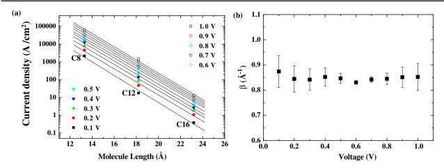
Figure 5. (a) A semilog plot of tunnelling current densities at different biases for three representative alkanethiol devices versus molecular length. The lines through the data points are exponential fittings. (b) Decay coefficient  $\beta$  values obtained from the slope of the exponential fittings as a function of the applied bias.
