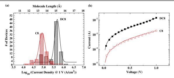
Figure 7. (a) Histogram of logarithmic current densities at 1 V for C8 and DC8 working devices. (b) I-V characteristics of C8 and DC8 representative devices. Symbols are experimental data and solid lines are fitting curves with the Simmons equation.
