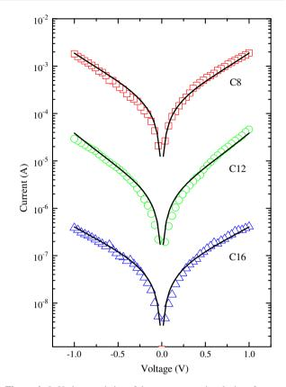
**Figure 4.** I-V characteristics of three representative devices for three different length alkanethiols (see text regarding the method used to select these representative devices). Symbols are experimental data and solid lines are curves fitted with the Simmons equation.
