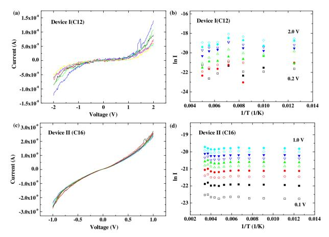
**Figure 6.** Examples of the temperature-variable I-V characterizations for two devices: Device I (C12) ((a), (b)) and Device II (C16) ((c), (d)). (a) I-V data at temperature from 200 to 80 K with a step of 20 K. (b) Arrhenius plot generated from the I-V data in (a) at voltages from 0.2 to 2.0 V with 0.2 V step. (c) I-V data at temperatures from 280 to 80 K with a step of 20 K. (d) Arrhenius plot generated from the I-V data in (c) at voltages from 0.1 to 1.0 V with 0.1 V step.
