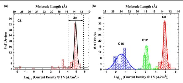
**Figure 2.** (a) Histogram of logarithmic current densities at 1 V for 'candidate' C8 molecular electronic devices. (b) Histograms of current densities at 1 V for 'working' C8, C12 and C16 devices. (See text for the definition of candidate and working devices.) Solid lines are Gaussian fitting curves.
