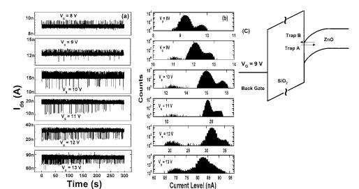
FIG. 3. (a) Raw drain current random telegraph signals for a time interval of 300 s observed in the ZnO nanowire FET at 4.2 K as a function of gate bias. The drain bias is kept constant at 2 V. (b) Histograms of the time-domain RTS data. The large and small peaks represent the empty or filled trap states, respectively. (c) Band diagram for back gate voltage at 9 V with two near interface oxide (border) traps.
