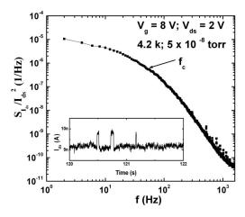
FIG. 2. Typical Lorentzian spectrum with corner frequency at  $\sim$ 18 Hz when the device is biased at  $V_{\rm g}$ =8 V and  $V_{\rm ds}$ =2 V; the inset shows the corresponding time domain RTS.
