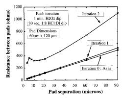
Fig. 4. Measured resistance vs pad separation for TLM structure with  $60 \, \mu \text{m} \times 120 \, \mu \text{m}$  pads on device layer. Curves are shown for (i) unetched sample (as deposited), after one etch iteration of approximately 2.5 nm, and after two etch iterations, with a total etch depth of approximately 5 nm. The change in resistance indicates a dramatic change in the sheet resistance between the contacts.
