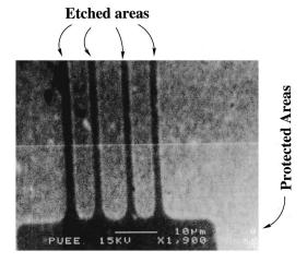
Fig. 3. Scanning electron micrograph of regions of GaAs patterned using wet chemical etching with stamped xylyl dithiol as etch mask.
